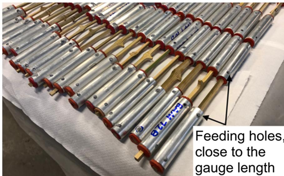
Fig. 3. Tension specimens.
